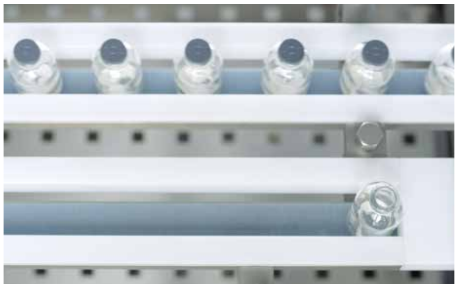
Vial rejection in case of incorrect first or second dosage
