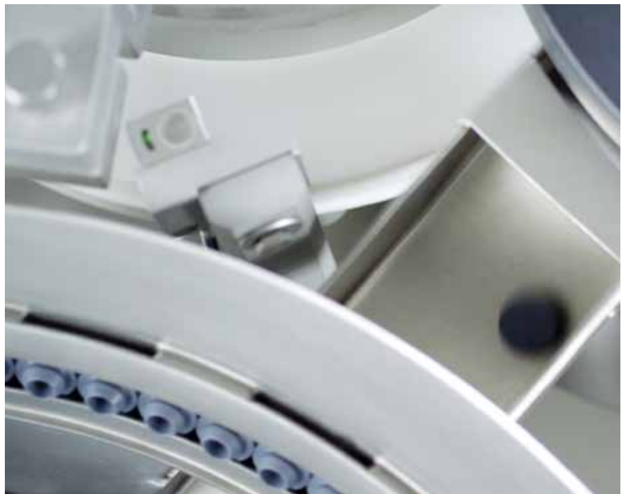
Stopper recovery in case of missing vial.
