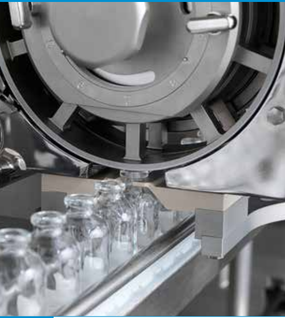
Dosing unit detail: vial neck centering device
