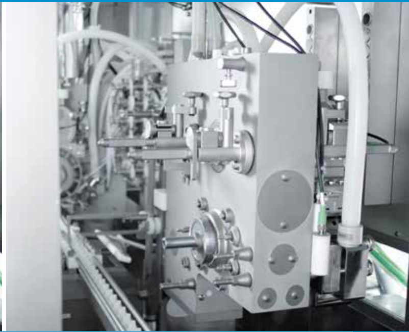
Dosing unit after removal of the dosing components
