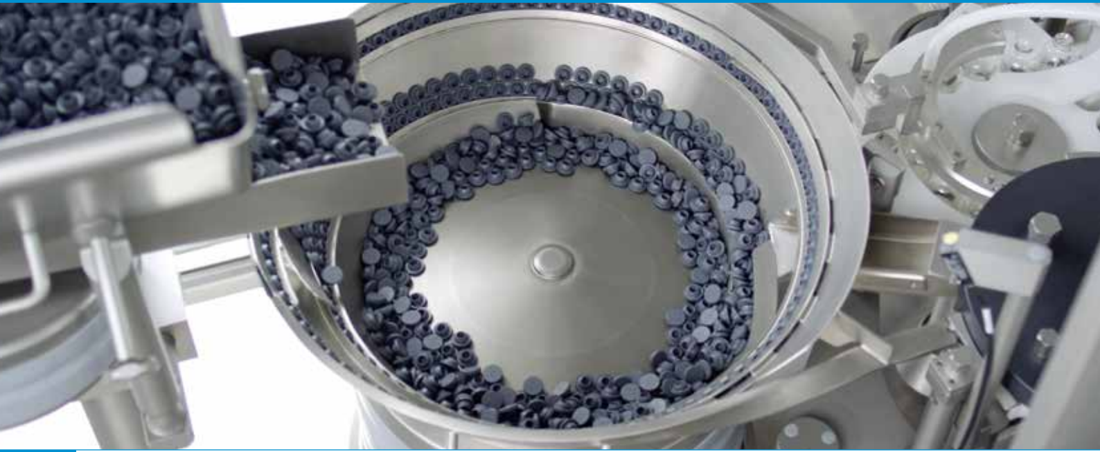
Stopper feeding by vibrating bowl
