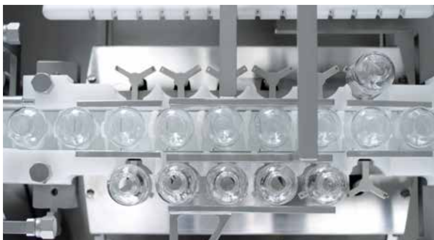
100% IPC gross weight sampling after first/second and/if present third dosing units
