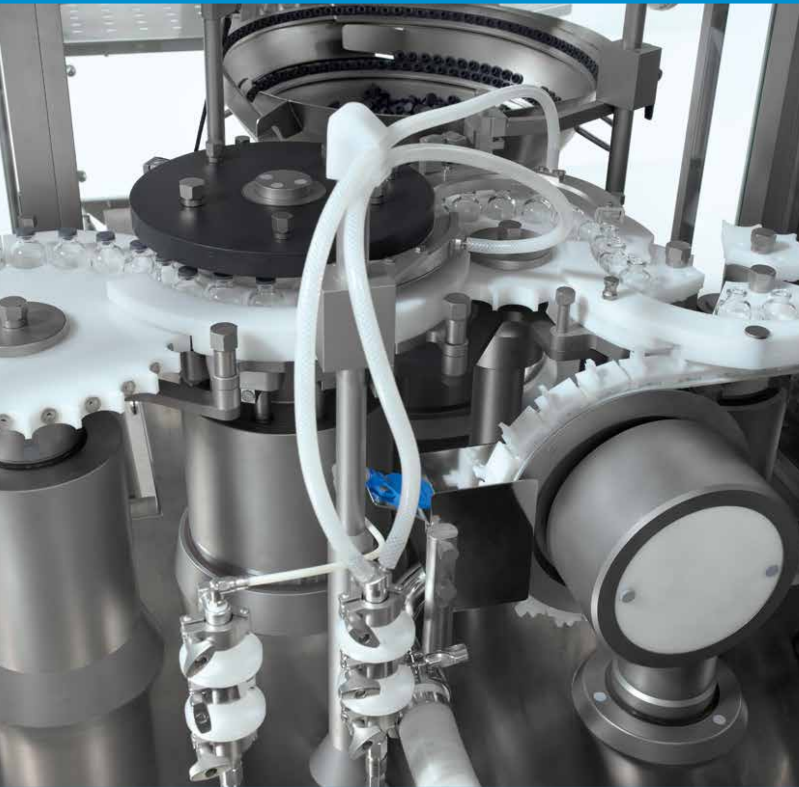
Xtrema gas purging station and powder cleaning device
